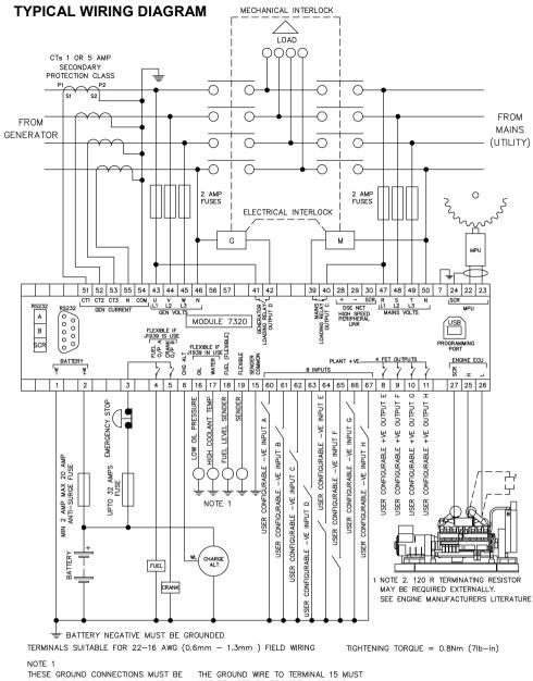
THESE GROUND CONNECTIONS MUST BE ON THE ENGINE BLOCK, AND MUST BE TO THE SENDER BODIES.
